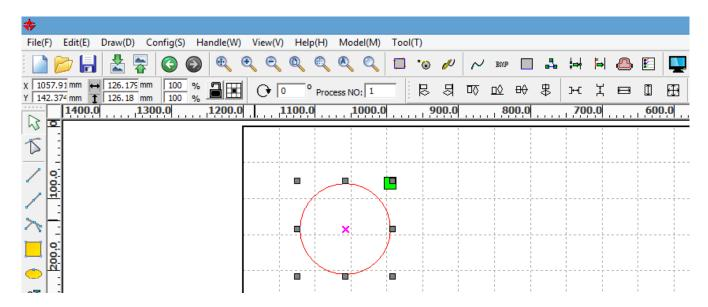
4.) The size of the circle can be changed by using the menu-bar tools. Locate the dimension menu in the upper left of the RDWorks software. The width of the circle can be modified by changing the numbers just left of the tool with left-right arrows. The height of the circle can be modified by changing the numbers just left of the tool with up-down arrows.
