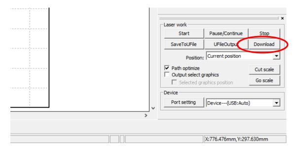
11.) The "Download" command will start a new connection to the laser machine. The "Name document" window will appear. Enter a name for the laser machine to use. The RDWorks software will only accept letters and numbers to be used for the Document name and is limited to a maximum eight characters long.
