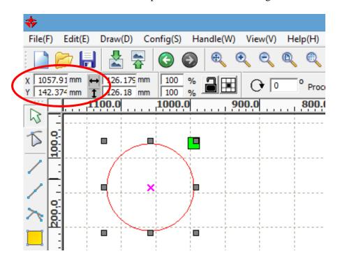
6.) Type in new values in the ↔ (Size in X dimension) and \$\(\) (Size in Y dimension) to change the dimensions of the ellipse. In this example, the dimensions are set to "10" millimeters.
