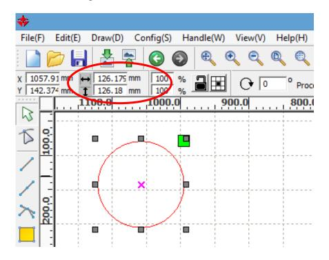
5.) The location of the circle can be changed by using the menu-bar tools. Locate the coordinate menu in the upper left of the RDWorks software. The X and Y values show the position of the circle in the Drawing Area. Change the X value to move the circle Upward or Downward. This relates to the Front and Back of the laser work table. Change the Y value to move the circle toward the left or right. Notice that the X and Y coordinates correspond to the ruler at the edge of the work area.
