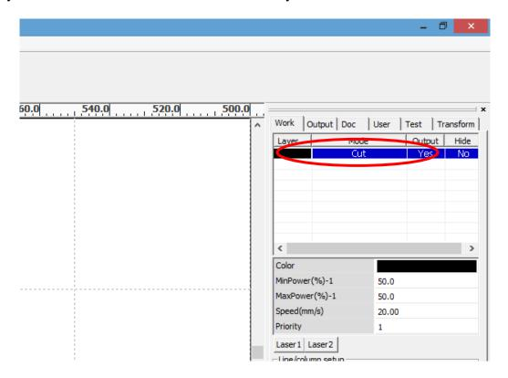
8.) After clicking on the layer, the "Layer Parameter" window will appear. Please refer to our "Common Settings for Cutting and Engraving Materials" data sheet for help finding the appropriate settings of the materials you are using. In this example the "Speed" has been set to "10", and the "Min Power" and "Max Power" were set to "70". Click "Ok" when done.
