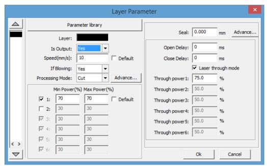
The "Through Power 1" is set to "75". This is the initial piercing power used when the laser starts cutting.
