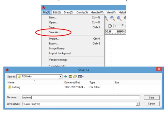
This file has been saved with the name "circletest.rld". The \*.rld file extension is for this RDWorks program and does not denote any other software file format.
